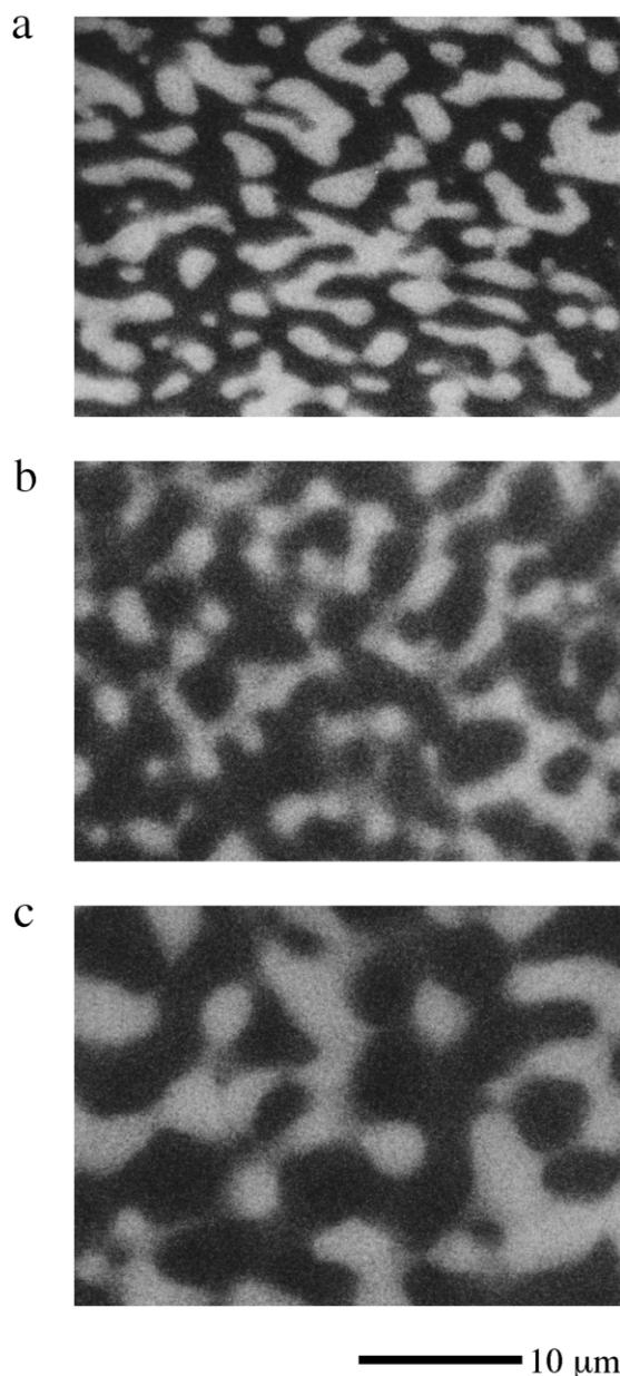
Fig. 2. Electron micrographs of microtomed surface of the blend undergoing phase dissolution at 155 °C for duration  $t$ . (a)  $t = 0$  s; (b)  $8.64 \times 10^4$  s; (c)  $3.456 \times 10^5$  s. Phase separation time at 180 °C  $t_{ps}$  is 6480 s.
