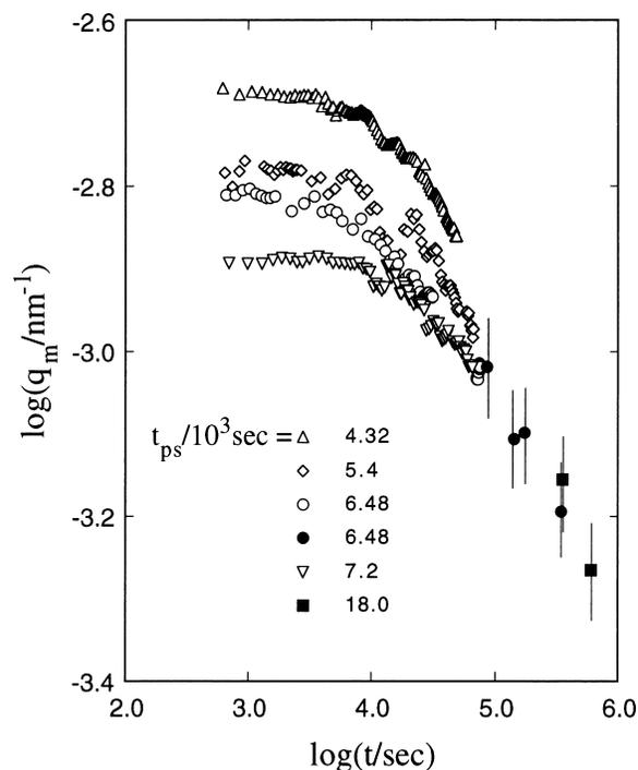
Fig. 3. Double-logarithmic plots of  $q_m$  against time  $t$  for various phase separation times  $t_{ps}$  at 180 °C. Filled symbols (●, ■) indicate  $q_m$  evaluated from image analysis of electron micrographs.
